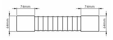
This 204 x 60 rectangular flexible bend is 500mm long and manufactured from white high impact polystyrene and PVC
