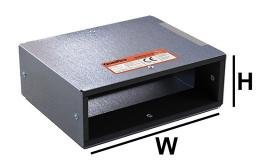
The rectangular fire sleeve range is designed to be built into the wall and sealed with intumescent mastic, available for 110x54, 204x60 & 220x90mm ducting
