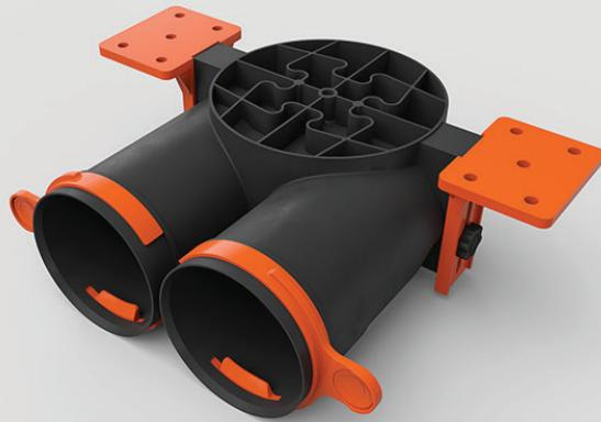
The low-profile plenum box AERO-PRO / SLIM BOX 2x75 allows for the installation of the ERGOVENT diffuser in just a 14 cm space (**fig. 3**). However, it is also fully suitable for installation in spaces up to 20 cm, as the box height can be adjusted using the side brackets (**fig. 4**). The plenum box is compatible with ERGOVENT RONDO-125, KVADRO-125, and other diffusers with a 125 mm connection.
